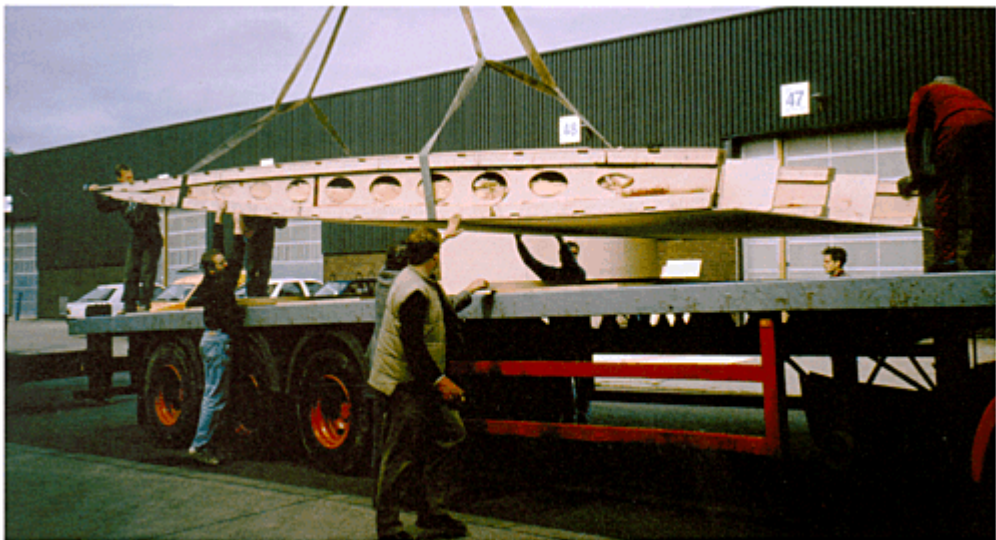
5.3 Transportation of prefabricated wing section
